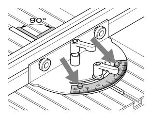
3. Retighten fixing screws.
